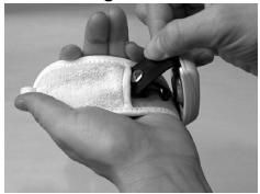
Slide the straps on the electronic module into the pockets on the front of the fabric headband.
