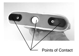
The elastic on the fabric headband is adjustable, and stretches to fit the head. The fabric headband may be detached for replacement or washing.
