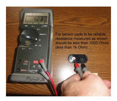
To make the measurement, first clean the sensor pad with alcohol or soap & water. Then touch one probe of the meter to the snap on the sensor pad being measured, and press the other probe into the middle of the rubber pad with about 8 ounces of force. Ohm meters may read out resistance in Ohms, or in kOhms (thousands of ohms).
