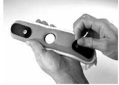
First remove the conductive pads by gently pulling around the rivet, and then remove the module. The conductive pads are made of specially engineered conductive medical silicone. Save these pads!
